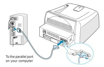
**3** Connect the other end of the cable to the parallel interface port on your computer, and tighten the screws.
